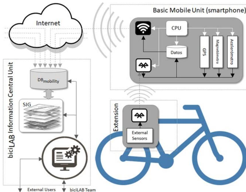
**Fig. 3.** Mobility data acquisition system as basic infrastructure of biciLAB.
